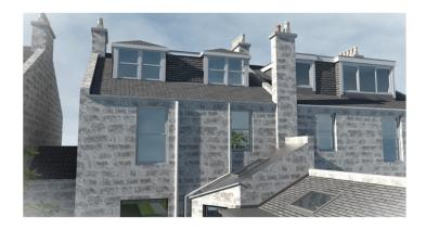
\* Revised proposal with the peaked traditional slated roof over each dormer and a mansard link panel between the two window, which is set back to soften the appearance.
